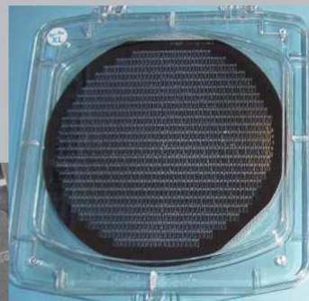
6-inch wafer with more than 1000 probes
