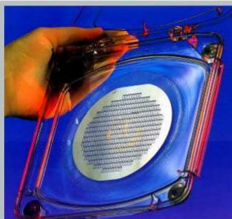
4-inch wafer with 388 probes
